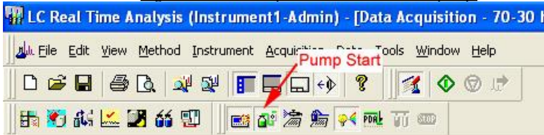
Fig. 4. Click the Pump On/Off icon to start the pump.
